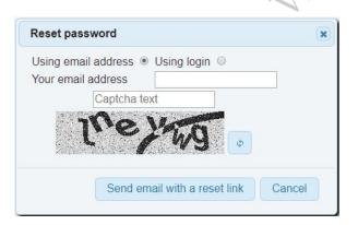
The reset password dialog will send an email that contains a link to reset the password. Two options are available input email address or login. The Captcha text has to be entered. If it is impossible to decipher it, use the refresh button to get an other one.
