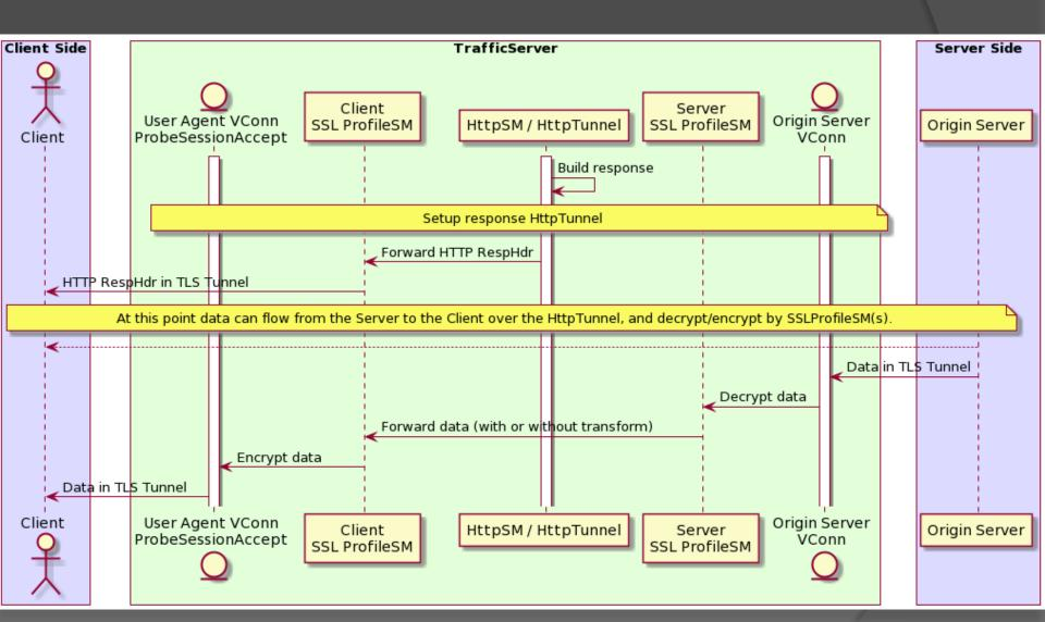
Handle SSL from Blind Tunnel with SslProfileSM
