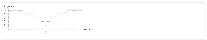
For 32-bit integers encoded using a "unsigned" variable length encoding, the histogram of int value to number of encoded bytes looks like this:
