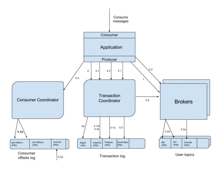
In the diagram above, the sharp edged boxes represent distinct machines. The rounded boxes at the bottom represent Kafka TopicPartitions, and the diagonally rounded boxes represent logical entities which run inside brokers.
